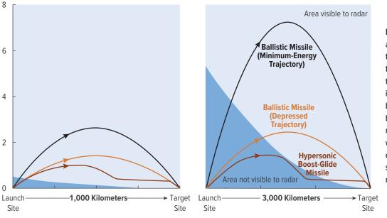
Because of its altitude, a ballistic missile would theoretically be visible to a radar located at the target site much earlier in its flight than a hypersonic boost-glide missile would be. To detect and track a missile, however, the radar would have to be powerful enough to generate a signal that would reach the missile.
